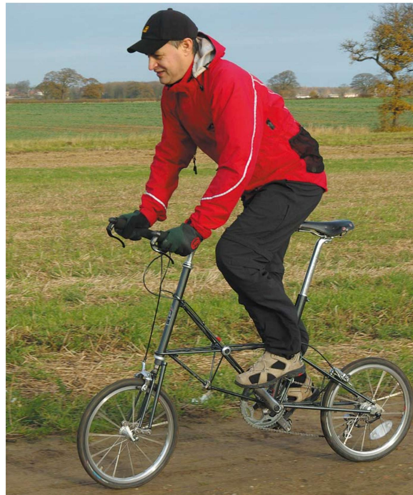
Both wheels are built with 24 spokes in the Moulton 17" (369) rim size, and are fitted with Schwalbe Stelvio 32 mm tyres. A nice touch is the offset spoke holes on the rear Velocity rim, which reduce the dish required and hence make a stronger wheel.
