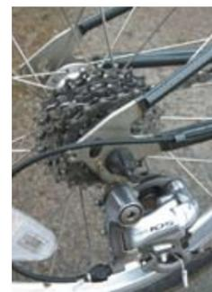
The Shimano Capreo 9-26 cassette gives a gear range of 33 to 96". Note also the unpainted stainless steel dropouts.
