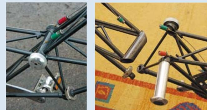
Separating the bike takes under a minute and no tools, leaving two relatively compact halves to stow.
